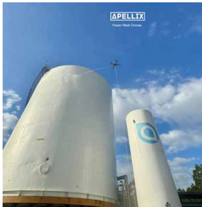
Today's Apellix systems deliver up to 4,000 PSI and up to 11 gallons per minute, reaching working heights of around 195 feet.
