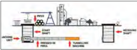
Figure 2: Microtunneling. Retrieved Jan. 9, 2026, from: https://m-konstruktor.com/steel-moulds-and-concrete-equipment/microtunneling-pipe-steel-moulds
