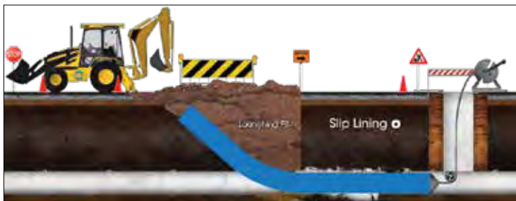
Figure 6: Sliplining. Retrieved Jan. 9, 2026, from: https://www.tuboseal.co.za/
